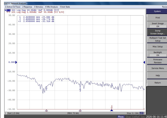
Output return loss vs frequency
