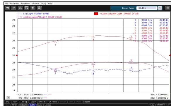
Gain compression at 10W out
