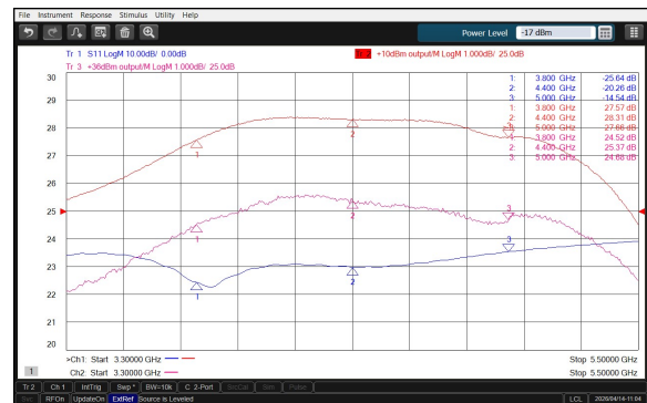
Gain compression at 4W
